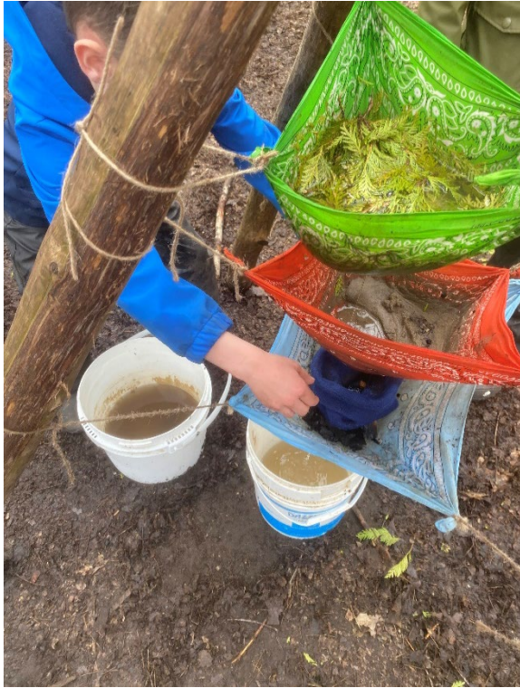
A close up of the tiered filtration system
